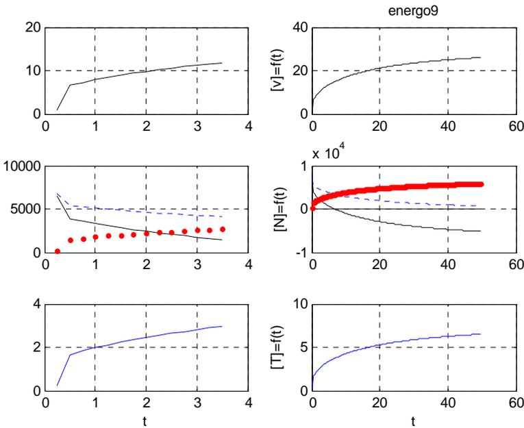
Fig. 1. the notations here are:  $v$  – the function found by integrating by (6.4),  $T$  – temperature, the function found on (3.12),  $N$  – functions of power reversible electromachines (a thin black continuous line), power of an environment (a thick red line), total power (a thin dark blue dotted red line). Right windows show all the time period starting till the maximal speed, and left windows – only its initial part.
